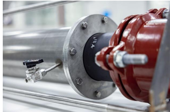
Figure 2. A test setup to measure the permeation through a PE pipe.
