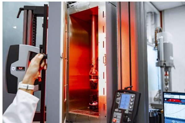
Figure 1. A universal tensile tester for SHT (in the background on the right a dynamic tensile tester for the CRB).
