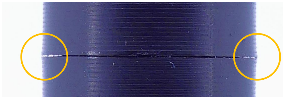
Figure 3. PE material will flow out as a result of the notching process (orange circles). This creates a small rim directly next to the notch.
