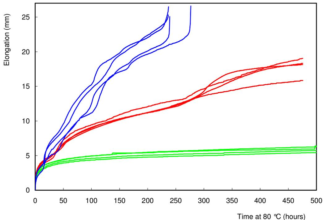
*Figure 3. Slow Peel Tests on joints made in pipes made of resin D (red), resin E (green) and resin F (blue). Each group shows the curves of 4 out of 12 test bars.*
