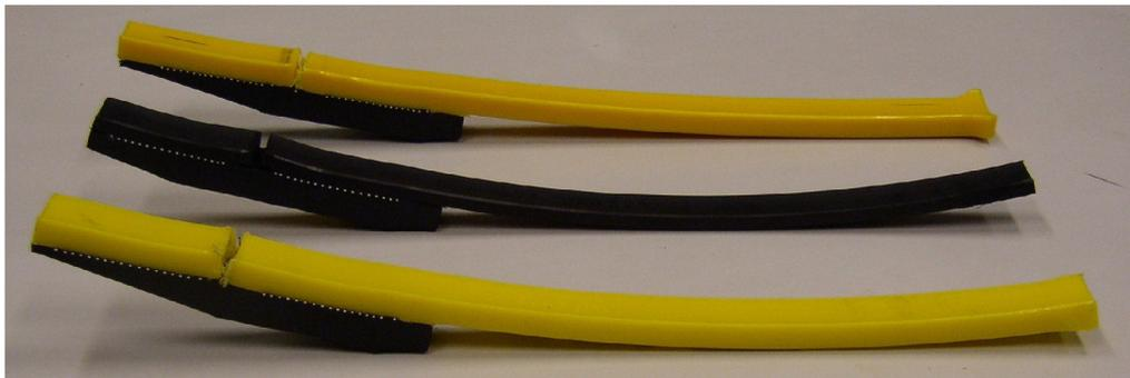
*Figure 1. Strips (20 mm wide) for the Slow Peel Test.*
