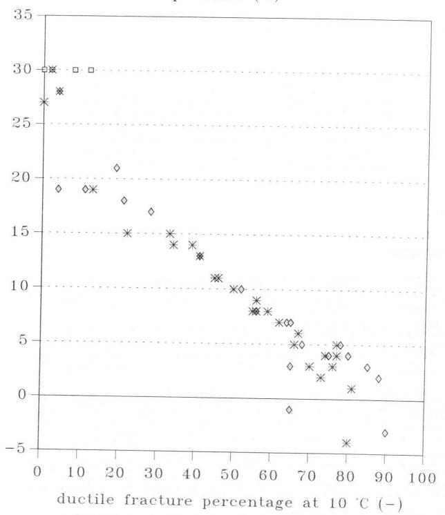
FIGURE 2: The transition temperature as a function of ductile fracture percentage at 10 °C. In the figure the following symbols are used:
