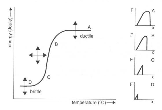
FIGURE 1: The fracture energy (Joule) as a function of the test temperature (main figure). In this main figure the codes A, B, C & D are given. Beside the main figure the force-deflection-(F-x) curves given at the locations of code A, B, C & D.
