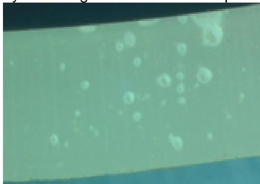
Figure 11 – Degradation of POM by HCl/H<sub>2</sub>O
