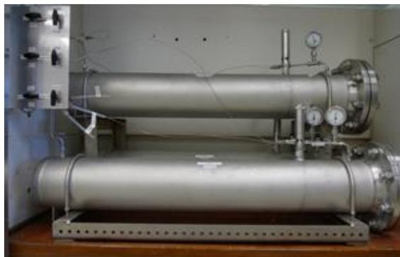
Figure 8 – Test rig configuration for high pressure applications (up to 8 bars)
