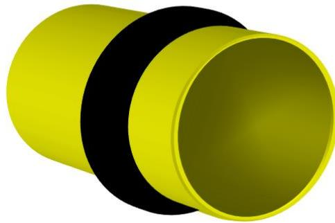
Figure 4 – Set-up for exposing stressed rubber rings to a particular gaseous environment
