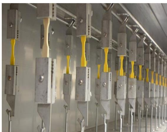
Figure 5 – Constant load experiments on PVC samples
