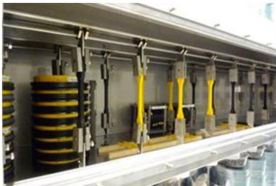
Figure 7 – Opened test rig with several ESC samples of PE and rubber
