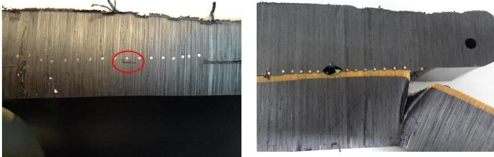
**Figure 6: Examples of different types of voids found with PAUT analysis**
