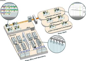
The verified pressure testing data in the Kiwa laboratory is sent directly to the Kiwa Online server. The customer can access via a secured and personal plug-in the latest data and project information through its Pipeson® Analyzer or DataManager software (more info see www.pipeson.com).
