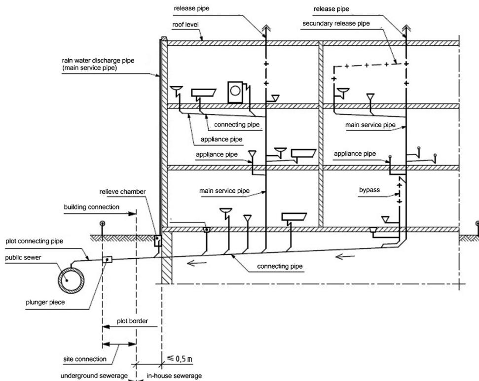
Figure 1 - Names of pipes
