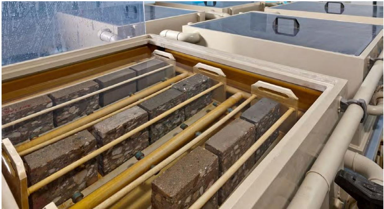
Figure 3 Test facility for storing the specimens in acid
