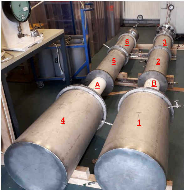
Figure 3. Overview of the test setup for two piping systems (A and B). Jacket pipes 1 and 4 contain the end fittings. Jacket pipes 2 and 5 contain the inline couplers. Jacket pipes 3 and 6 contain the pipe itself.
